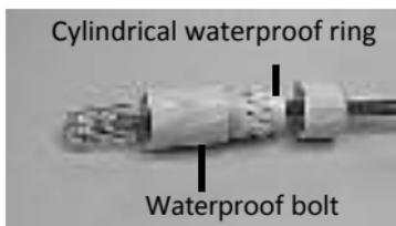
4. Insert the cable into the Ethernet copper interface and screw the waterproof bolt in.
