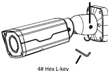
5. Mount your camera onto the wall and connect all cables.
