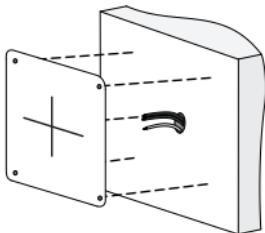
**2** Lead the cables across the hole on the wall.
